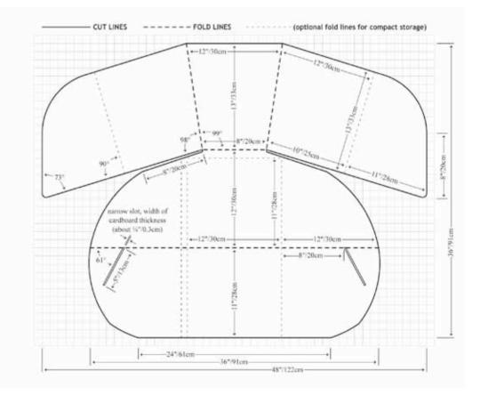
the 76° angled corners from the back panel fit snugly to hold up the front panel.
